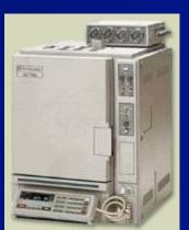
■Air sampled from the chamber was analyzed by **SHIMADZU GC-14b** gas chromatograph at flame-ionization detector. Methane emission was calculated from concentration rise within the chamber.
