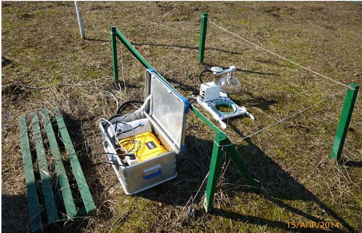
LI-8100a - Automated Soil CO<sub>2</sub> Flux System with clear long-term chamber installed at Lower Observation Point (IMCES).
